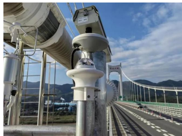
Fig 3. Installation of Beidou High-Precision Monitoring Station Equipment
