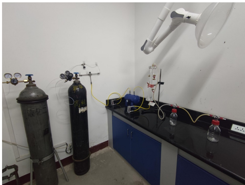
Fig 2. Laboratory-scale simulated industrial wet desulfurization unit
