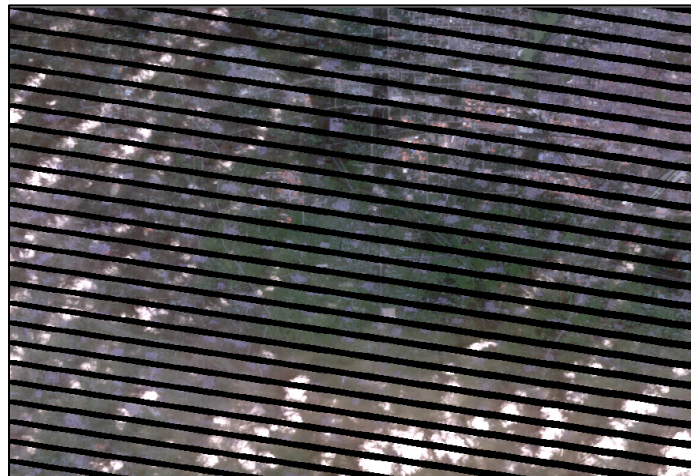
Figure 3. Stripe defect image
