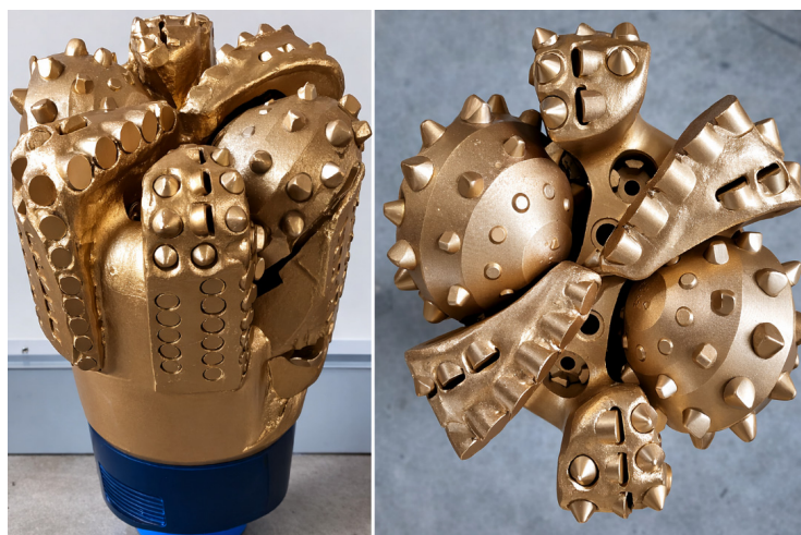
Fig 9. Schematic diagram of a PDC–roller-cone hybrid drill bit with an independent buffering structure
