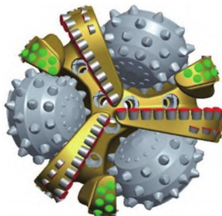
Fig 7. “3+3+3” configuration hybrid drill bit with an independent buffering structure
