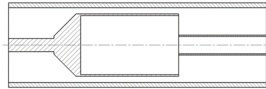
Figure 5. Simplified diagram of the structure of the novel sand-bailing device
