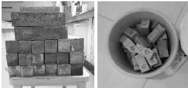
Fig 6. Flexural and compressive specimens of carbon nanotube cement matrix composites
