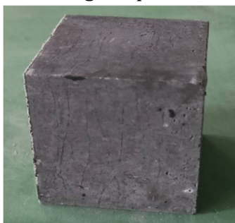
Fig 3. Geopolymer solidified body based on fly ash
