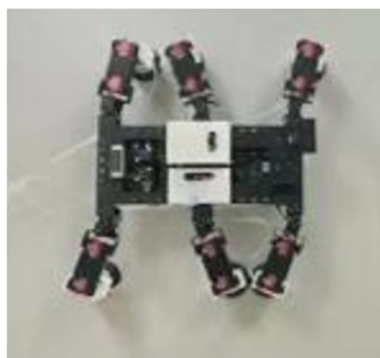
Figure 4. Negative-pressure suction robot
