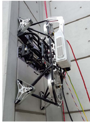
Figure 8. Rope-driven climbing robot
