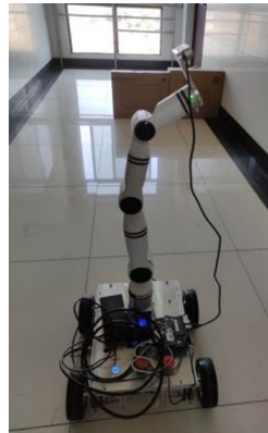
Figure 9. Compact mobile welding robot
