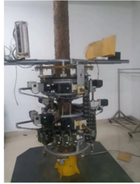
Figure 3. Ring-clamp climbing robot
