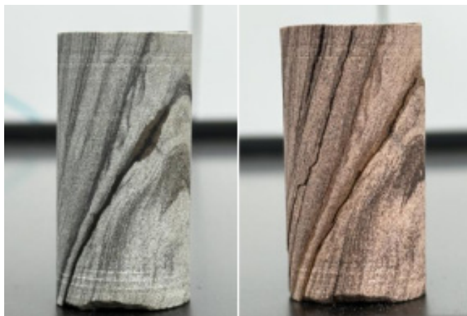
Figure 3. Comparison between Rock Heated to 1000°C and Untreated Rock
