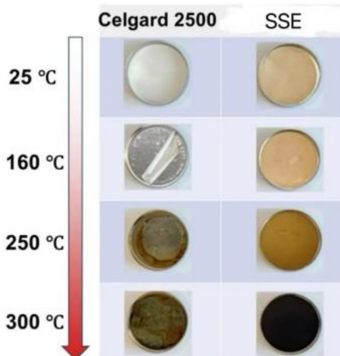
Figure 4. Comparison of thermal shrinkage between Celgard 2500 separator and ZIF-8 based SSE membrane
