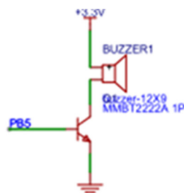
Figure 7. Buzzer Alarm Circuit
