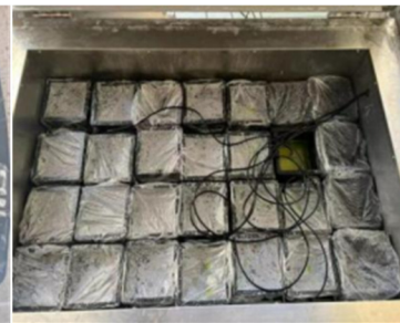
Fig 4. Asphalt placed in freeze-thaw cyclor
