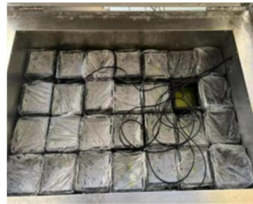
Fig 4. Asphalt placed in freeze-thaw cycler
